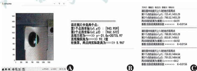
图 2 像素实际距离换算方法 A:通过实际距离计算出 2 个点间坐标 B:计算出 2 个点连线的直线方程,可知直线倾斜的角度为 92.7°,2 个点间实际距离为 5.967 mm C:多次在 1 mm 线段的两端取点,最后得出 1 mm 像素距离为 64.9,进而得出换算系数为 0.015 4 Figure 2 Conversion method of pixel to actual length A: The coordinates between the two points could be calculated through the actual length of the two coordinates B: The straight line equation determined by two coordinates was calculated. It was known that the angle between the two coordinates was 92.7°, and the actual distance between the two coordinates was 5.967 mm C: The coordinates were taken at 1 mm line segment several times, and the final pixel distance at 1 mm was 64.9, and the conversion coefficient was 0.015 4
